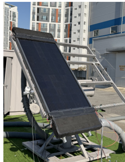
Fig. 4. Standard performance test of air-type PVT collector
