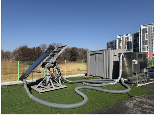
Fig. 5. Standard performance test of air-type PVT collector
