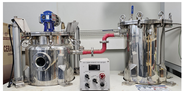
Fig. 5. Cl and K removal reactor
