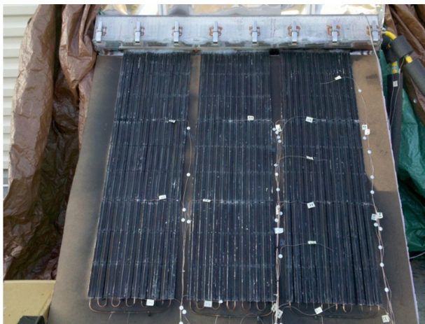
Fig. 4. Solar panels and heat exchanger. Selective black paint was applied to the surface of the panels. Thermocouples were attached to the positions indicated in Fig. 2. The glass and edge walls were not installed at this point.
