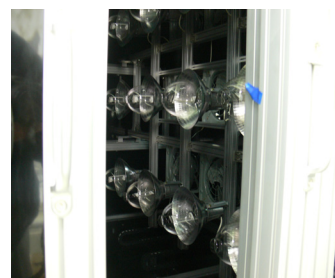
Fig. 5. Light soaking test equipment in test laboratory
