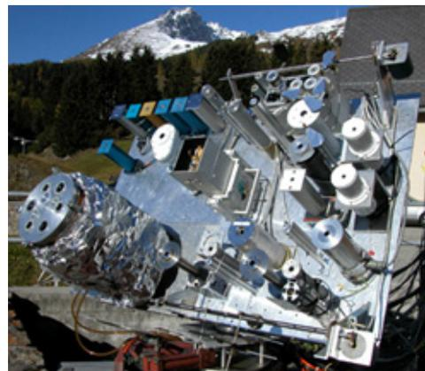
Fig. 1. Absolute cavity radiometer comparison to the WRC (Source: <http://www.pmodwrc.ch>)
