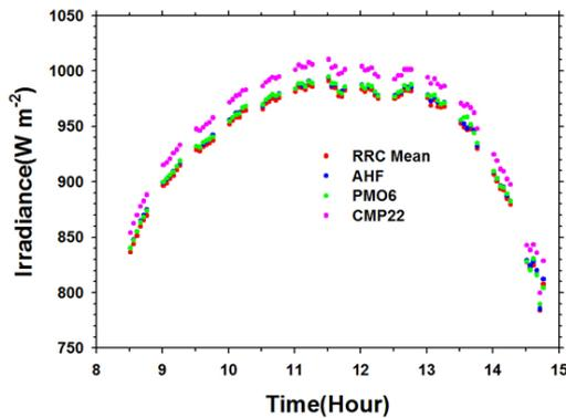
Fig. 6. Time series of solar radiation for RRC mean and Korea instruments (AHF, PMO6, CMP22) on 31 January 2012 (red point: mean of RRC standard instruments, blue point: AHF, green point: PMO6, and pink point: CMP22)
