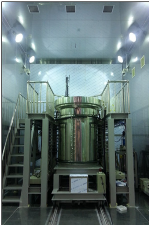
Fig. 13. Korea In-situ Production Experimental Device (KIPED), a 3D n-scale gas hydrate experimental device
