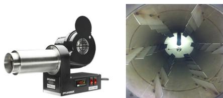
Fig. 4. Air blow Heater and inner part of the drum
