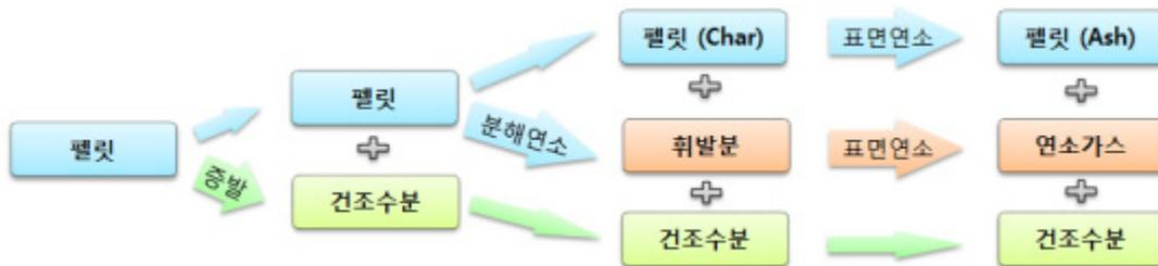
Fig. 2. Combustion reaction step for wood pellet<sup>[2]</sup>
