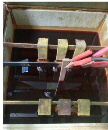
Fig. 4. Black chrome plating for surface treatment
